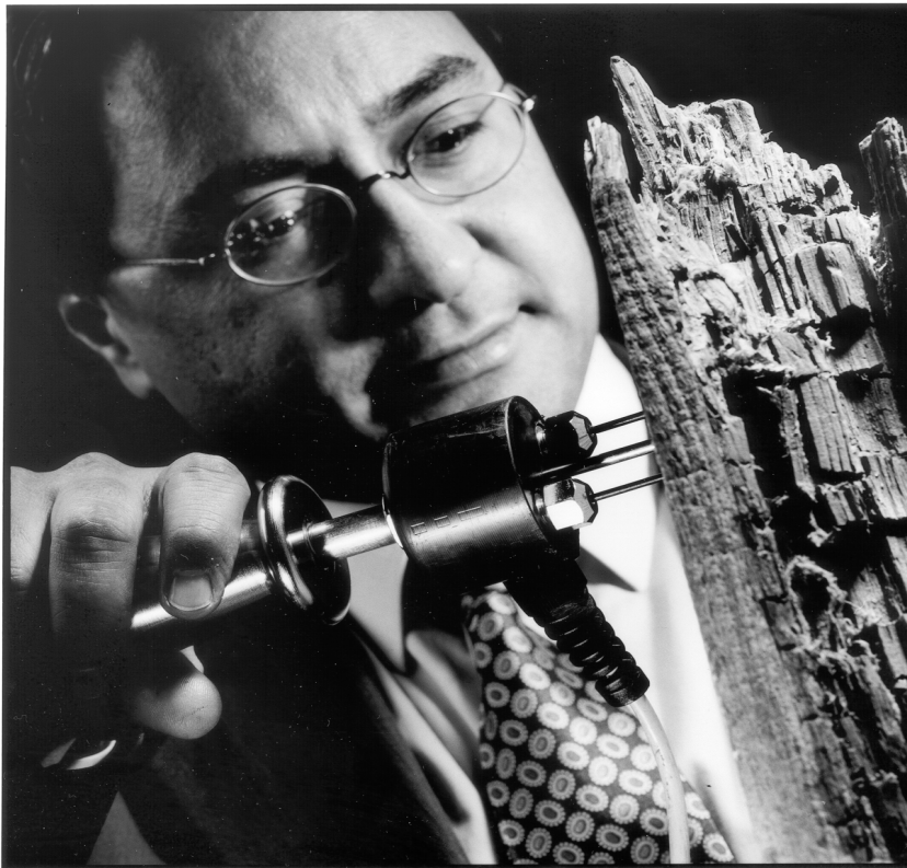
Dr Jagjit Singh using hammer probe to measure deep moisture content of timber.
